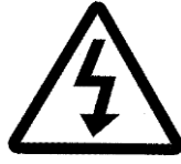
Danger!: High Voltage
