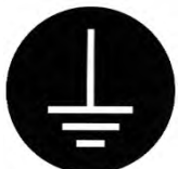
Connect grounding wire
